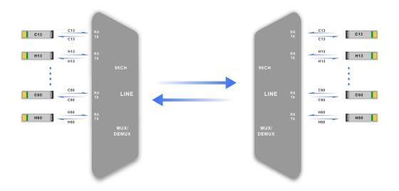
96 Channels DWDM MUX DEMUX, supports 96 channels difference business in two optical fiber for point-to-point transmission.
