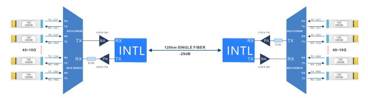
40CH DWDM MUX/ DEMUX Single fiber BIDI transmission
