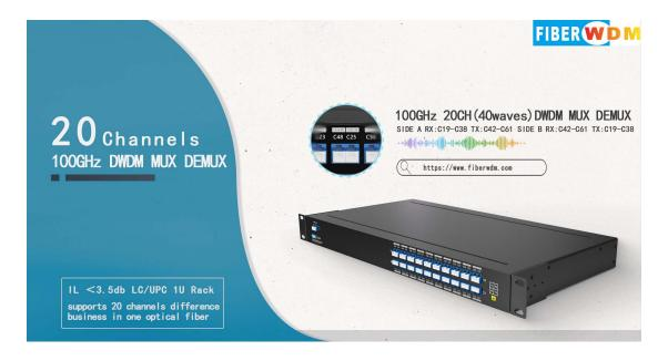
The 20ch(40waves) DWDM MUX/ DEMUX is used in pairs, designed by FIBERWDM, in side A, the waves are: RX C19 to C38(1562.23nm~1546.92nm), TX C42 to C61(1543.73nm~1528.77nm); And in side B, the waves are: RX C42 to C61(1543.73nm~1528.77nm), TX C19 to C38(1562.23nm~1546.92nm).
