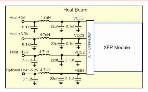
Recommended Host Board Power Supply Circuit
