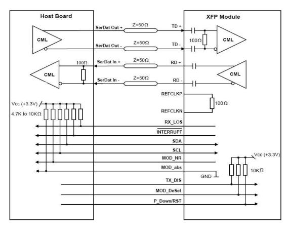
**Recommended High-speed Interface Circuit**
